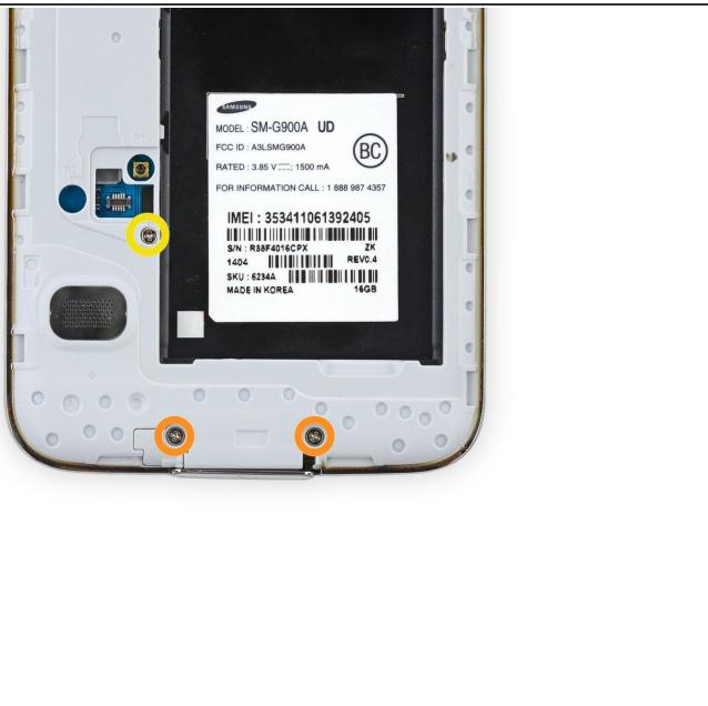
ⓘ Flip the phone over and remove the following screws from the battery side of the midframe:
