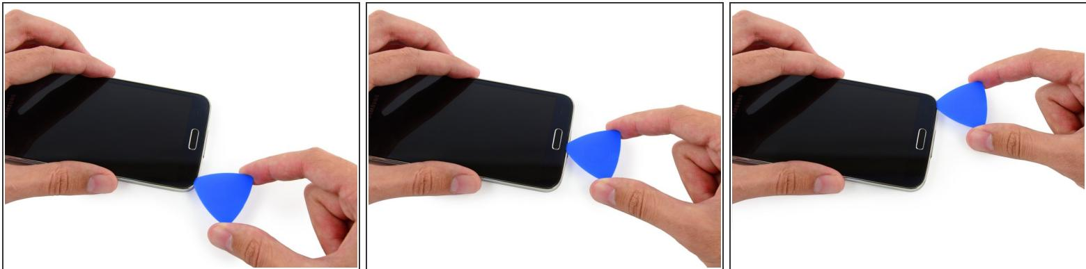
**⚠** The bottom end of the phone contains the soft button and home button ribbon cables. If you insert the opening pick too far into the phone you risk cutting these cables.
